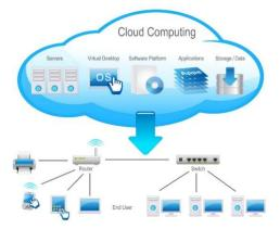
The main enabling technology for cloud computing is virtualization. Virtualization software separates a physical resource into one or more "virtual" resources, each of which can be easily used and managed to perform computing tasks. Cloud network is one such resource and is virtualized through multiple logical constructs and SW layers. It is essential to monitor cloud network to ensure transparency, correct and efficient operations, both from the customer and from the provider perspectives.
